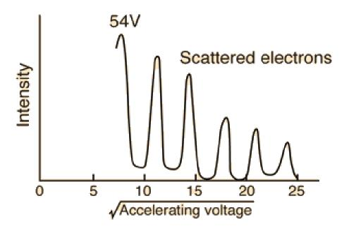
The experimental data above, reproduced above Davisson's article, shows repeated peaks of scattered electron intensity with increasing accelerating voltage. This data was collected at a fixed scattering angle. Using the Bragg law, the <u>deBroglie wavelength</u> expression, and the kinetic energy of the accelerated electrons gives the relationship
